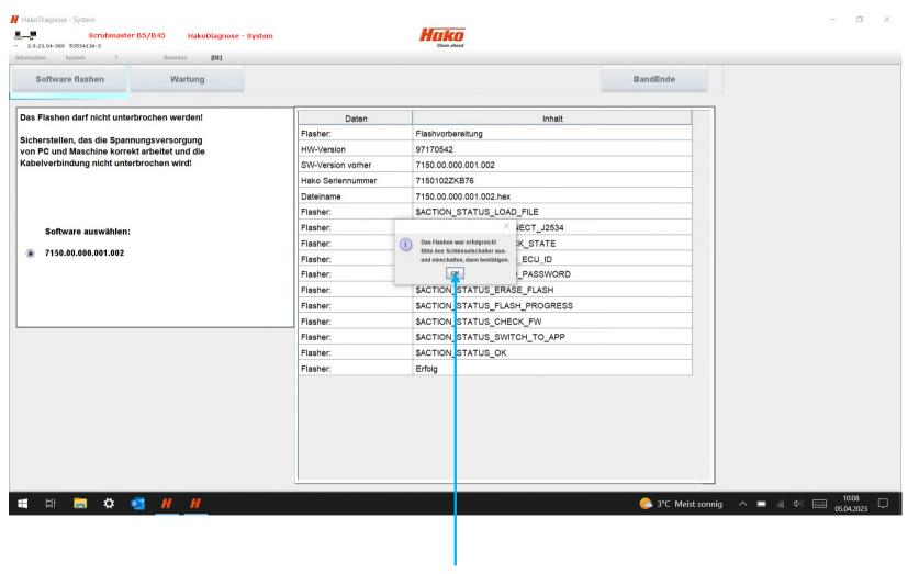
Flash process is succesfully finished. Switch off the machine, then confirm with "OK".
