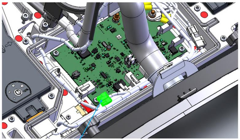
Connect plug A20 (fleet recorder) [is below the cable from X7] with adapter plug Microfit (to A20) on OBD
