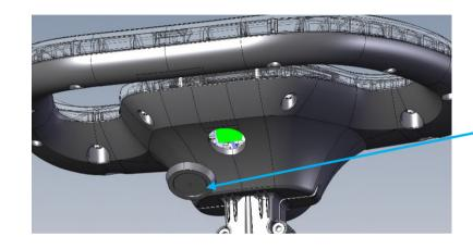
Diagnose plug cap press in the middle for secure fastening
